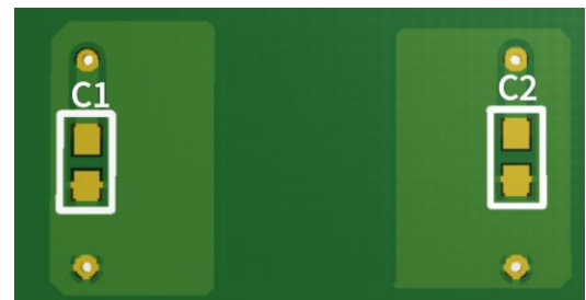
Figure8.3 Recommended PCB Layout — Bottom
