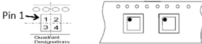
Figure 10.4 Quadrant Designation for Pin1 Orientation in Tape
