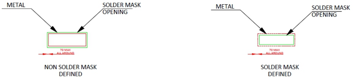
Figure 9.2 SOW8 Package Board Layout Example
