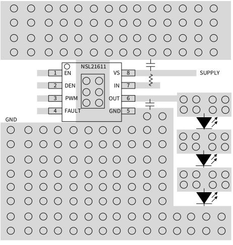
Figure 9.2 Example Layout Diagram for NSL21611
