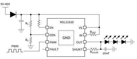
Figure 7.3 NSL21610 PWM Control LED Brightness Dimming
