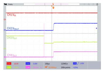
Figure 6.6 Open-Load Protection Recovery
