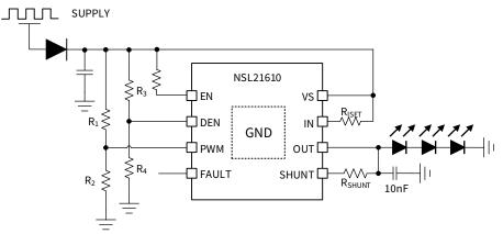
Figure 7.4 NSL21610 Power Supply Control LED Brightness Dimming
