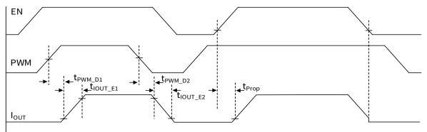
Figure 6.13 Start up sequence & PWM dimming timing
