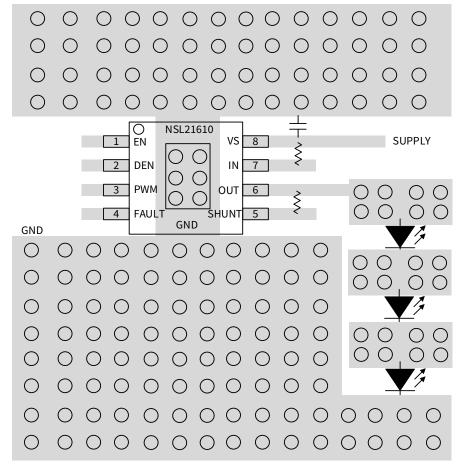
Figure 9.1 Example Layout Diagram for NSL21610
