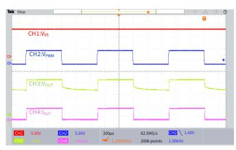
Figure 6.3 PWM Dimming at 1kHz
