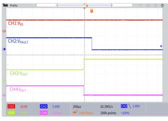
Figure 6.5 Open-Load Protection
