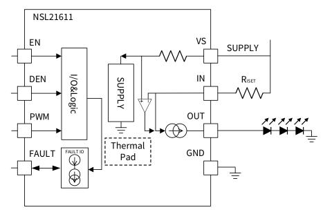
Figure 7.2 NSL21611 Block Diagram
