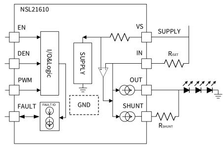
Figure 7.1 NSL21610 Block Diagram
