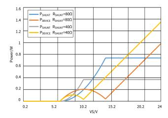
Figure 6.12 Power Dissipation vs Supply Voltage (Iset=99mA)
