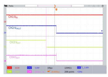
Figure 6.7 LED Short-to-GND Protection
