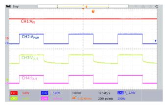
Figure 6.4 PWM Dimming at 200Hz
