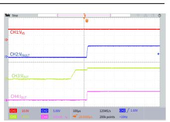
Figure 6.8 LED Short-to-GND Protection Recovery
