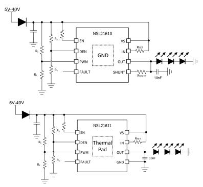
Figure 8.1 Simple Application Without MCU
