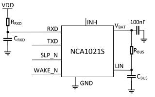
Figure 6. 1 Timing test circuit for LIN transceiver
