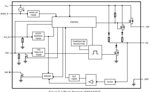
Figure 7. 1 Block diagram of NCA1021S
