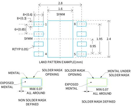
Figure 9. 4 DFN8 package board layout example
