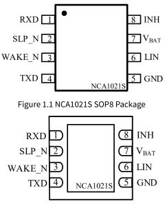
Figure 1.2 NCA1021S DFN8 Package
