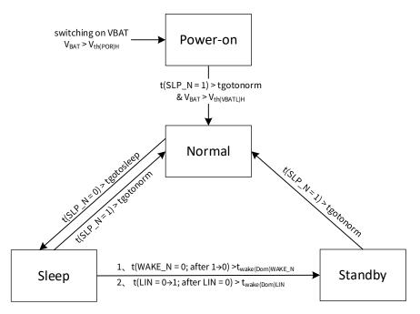
Figure 7. 2 State diagram of NCA1021S
