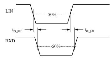
Figure 6. 4 Propagation delay and transition times from LIN to RXD
