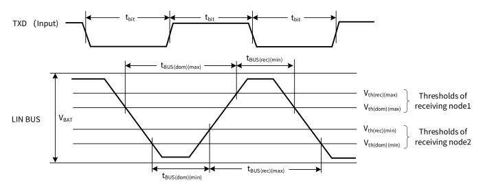
Figure 6. 2 Timing diagram of LIN transceiver
