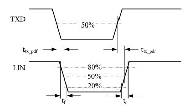
Figure 6. 3 Propagation delay and transition times from TXD to LIN
