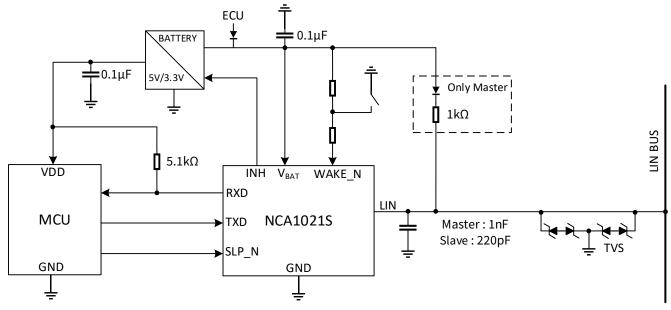
Figure 8. 1 Basic schematic of NCA1021S
