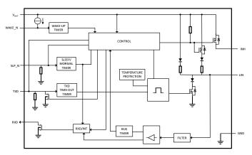
Figure 1. NCA1021S block diagram
