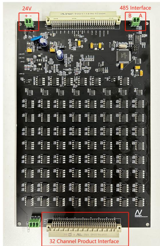
Figure1.1 NSx2860/9260 evaluation board Top View
