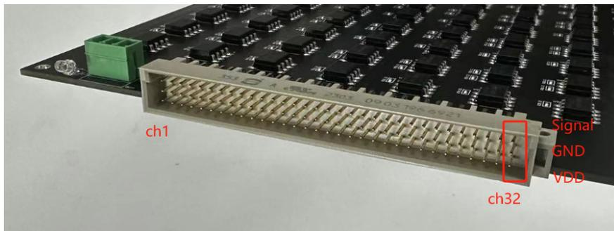
Figure 1.2 NSx2860/9260 MUL CAL SYSTEM 32 Channel Product Interface
