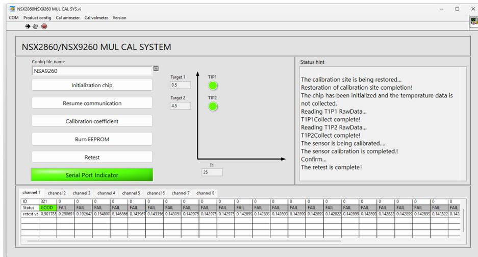
Figure 2.8 Retest Chip & Confirm
